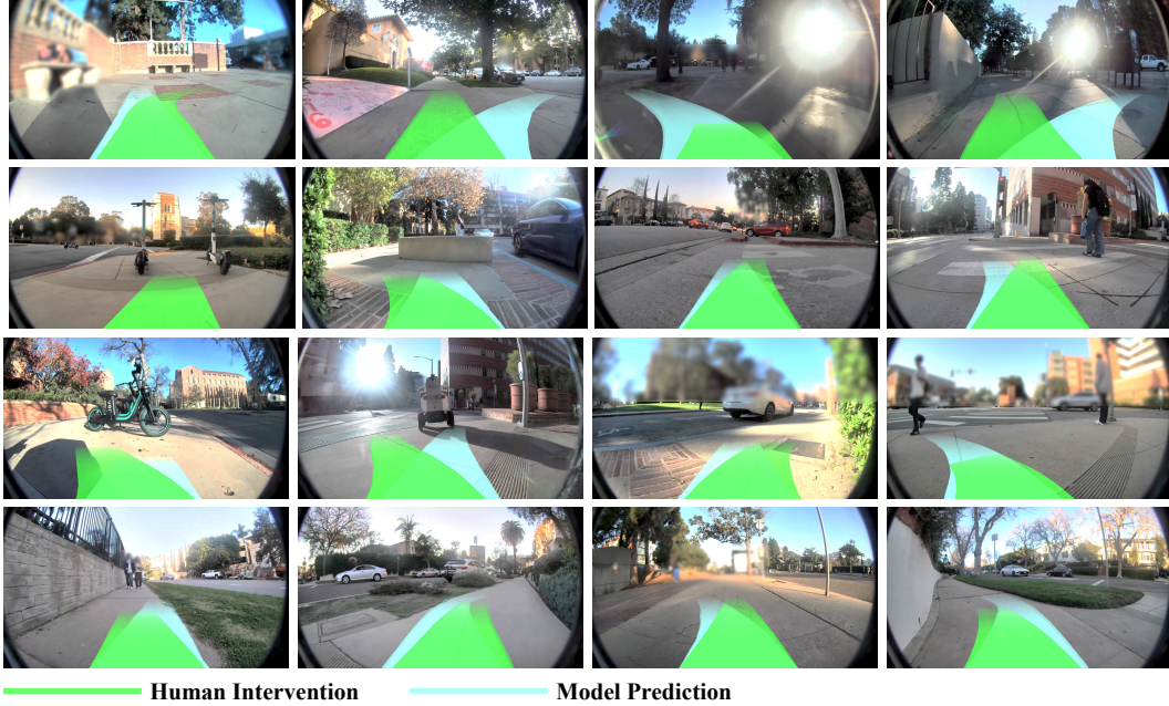
Figure 18: Qualitative comparison between FlowPilot predictions and human interventions. We visualize representative real-world frames with the model-predicted path (cyan) and the trajectory executed during human intervention (green). Across diverse sidewalk scenes, the intervention traces highlight where humans deviate from the model to ensure safety and progress.
