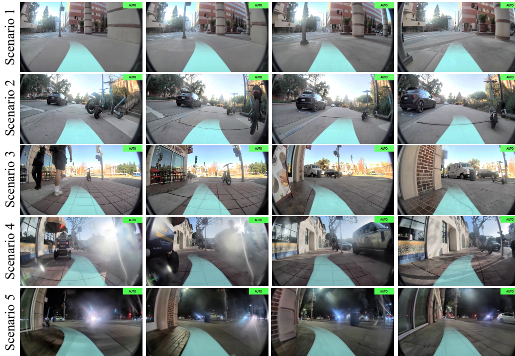
Figure 13: Reactive obstacle avoidance in cluttered sidewalks. FlowPilot selects safe bypass maneuvers around static obstacles and returns to the nominal path after passing them.
