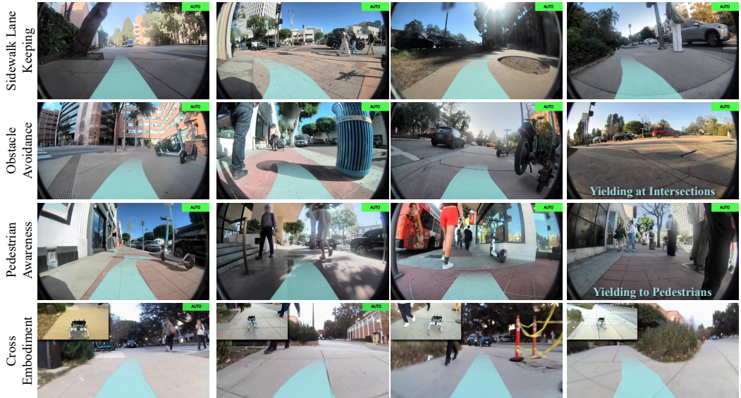
Figure 8: Qualitative results in diverse real-world sidewalk environments. We visualize the trajectories predicted by FlowPilot and executed by the robot during real-world deployment.
