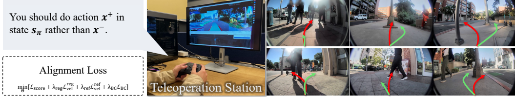
Figure 4: Preference alignment with human intervention for a specific robot. Human monitors policy predictions and intervenes when inappropriate behaviors occur. The corrective action x^+ is treated as preferred over the policy action x^- , providing pairwise feedback for alignment.
