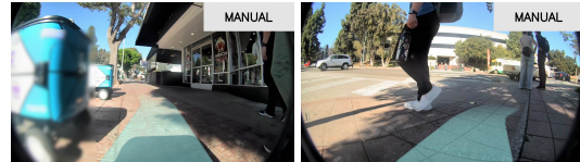
Figure 15: Representative failure cases in crowded or constrained scenes. When faced with ambiguous right-of-way or insufficient clearance, FlowPilot may be overly conservative and stop, requiring human intervention to continue.
